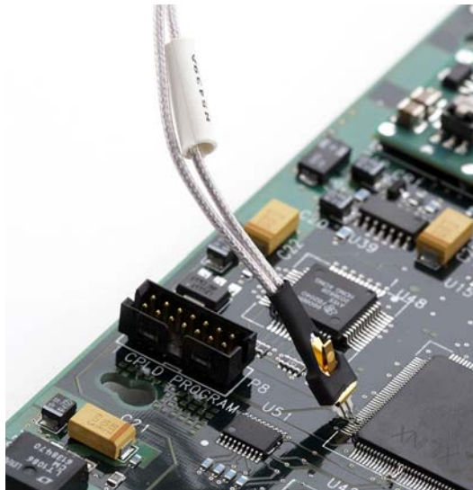
Figure 29 InfiniiMax III ZIF probe head connected to ZIF tip at more of a perpendicular angle than shown in Figure 28
