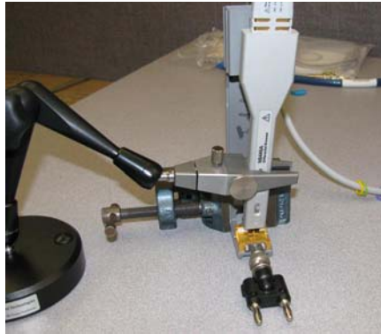
Figure 64 Setup for Measuring Input Resistance for Browser Probe Head
