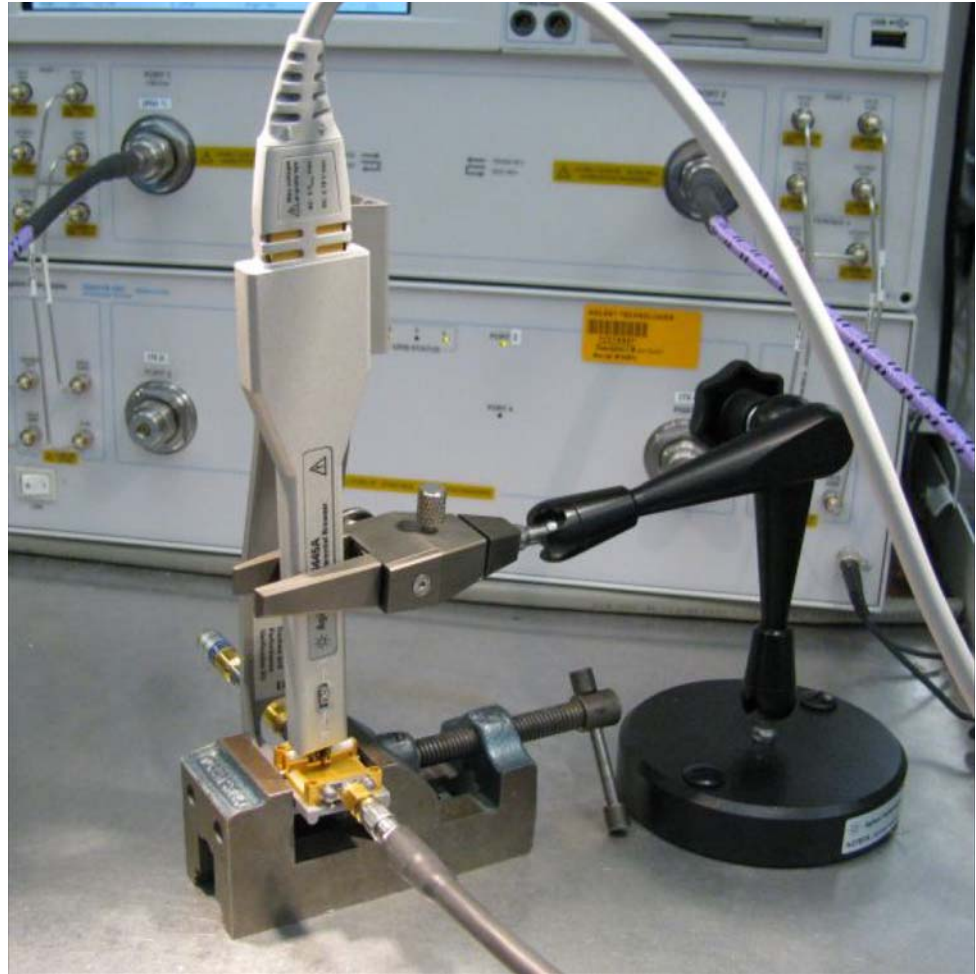
Figure 61 N2787A 3D Probe Positioner used to measure the N5445A browser with the N2803A amp
