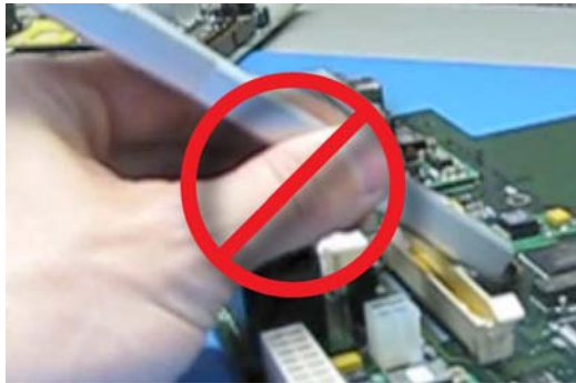
Figure 14 Improper Probe Handling
