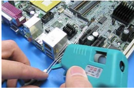
Figure 26 Using low-temperature hot glue to secure a probe head
