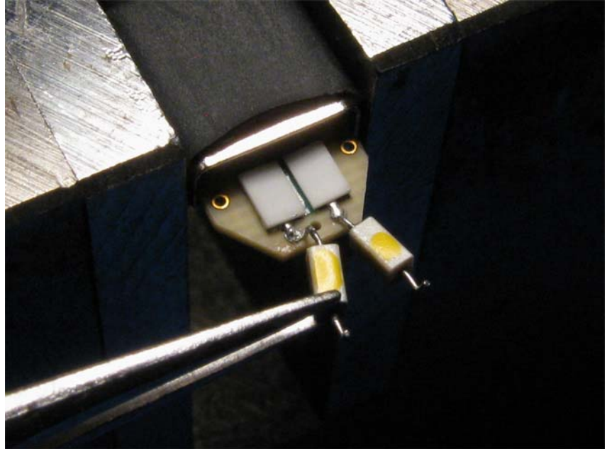
Figure 35 Soldering in a new axial resistor
